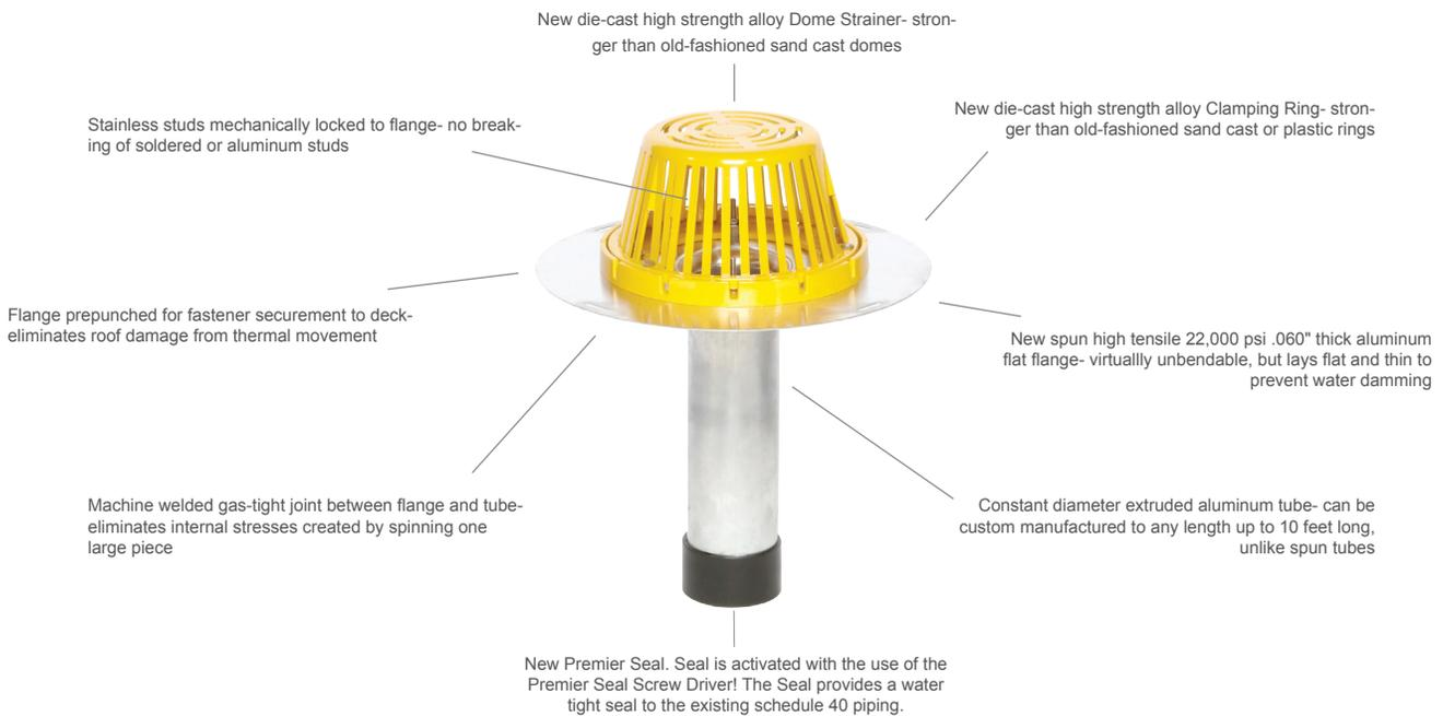
**New die-cast high strength alloy Dome Strainer** means fewer debris-clogged drain lines due to broken domes. Further, the Dome Strainer bolts down to prevent malicious vandalism to the drain system.
