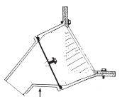
Outlet hub may be used at 45° or 90° by removing two bolts and changing outlet position one half rotation.
