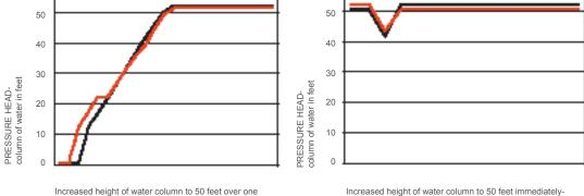
Increased height of water column to 50 feet over one SURGE: No leakage at seal Held pressure at a 50 feet water column for 18 hoursminute- No leakage at seal STATIC: No leakage at seal PVC DRAIN PIPE
