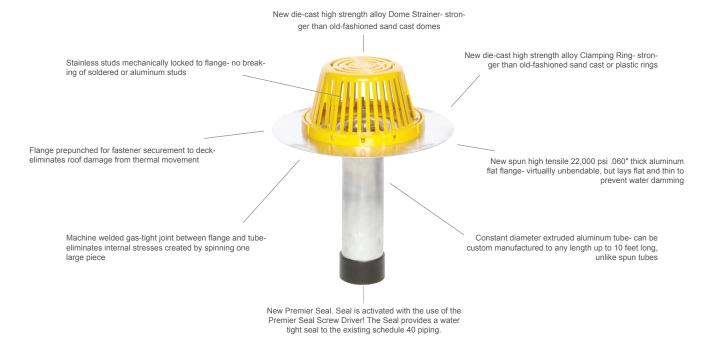
New die-cast high strength alloy Dome Strainer means fewer debris-clogged drain lines due to broken domes. Further, the Dome Strainer bolts down to prevent malicious vandalism to the drain system.
