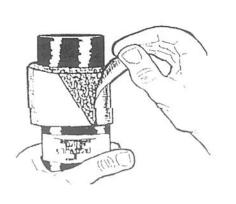
NOTE: Heat and U.V. will accelerate the expansion rate of the foam tape. In colder weather a heat gun may be used to expand foam tape. In the event that the precompressed tape has expanded larger than the inside diameter of the roof drain, the tape can be recompressed by hand.
