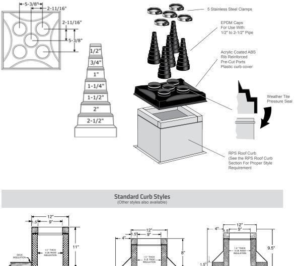
RC-2A For Decks with Lightweight Fill or Tapered Insulation
