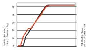
Increased height of water column to 50 feet over one minute- No leakage at seal
